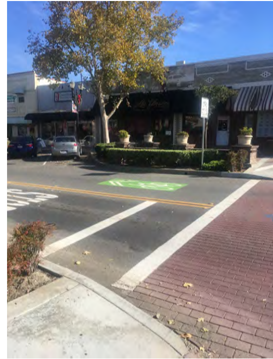
Downtown contains many features that have been shown to increase pedestrian comfort, and may be emulated elsewhere, such as bulb-outs, shown.
