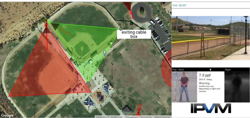
The Axis P1435-LE is 1080p resolution, at 53.00° AoV of its 35° to 95° range, delivers 7.3 PPF at 264.05' wide scene, 265ft - 10in from the camera.
