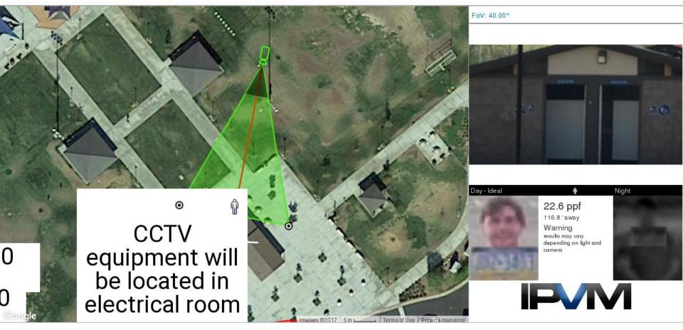
The Axis P1435-LE is 1080p resolution, at 40.00° AoV of its 35° to 95° range, delivers 22.6 PPF at 85.02' wide scene, 117ft - 10in from the camera.
