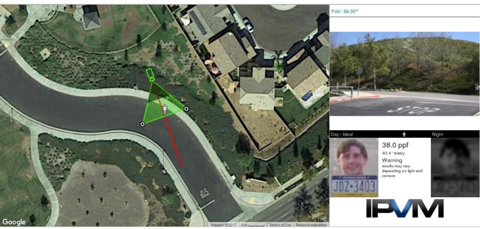
The Axis P1435-LE is 1080p resolution, at 64.00° AoV of its 35° to 95° range, delivers 38.0 PPF at 50.49' wide scene, 40ft - 5in from the camera.
