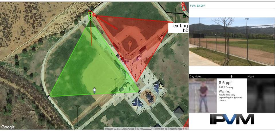
The Axis P1435-LE is 1080p resolution, at 63.00° AoV of its 35° to 95° range, delivers 5.6 PPF at 345.86' wide scene, 282ft - 2in from the camera.
