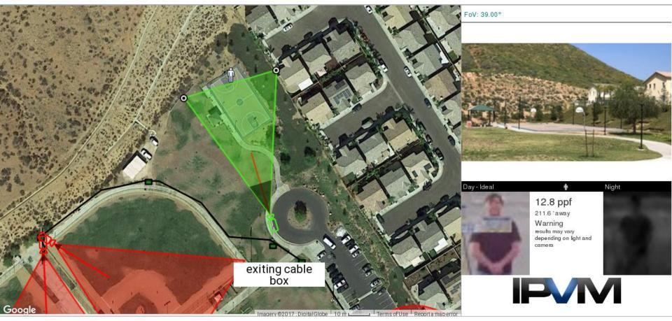
The Axis P1435-LE is 1080p resolution, at 39.00° AoV of its 35° to 95° range, delivers 12.8 PPF at 149.86' wide scene, 212ft - 7in from the camera.
